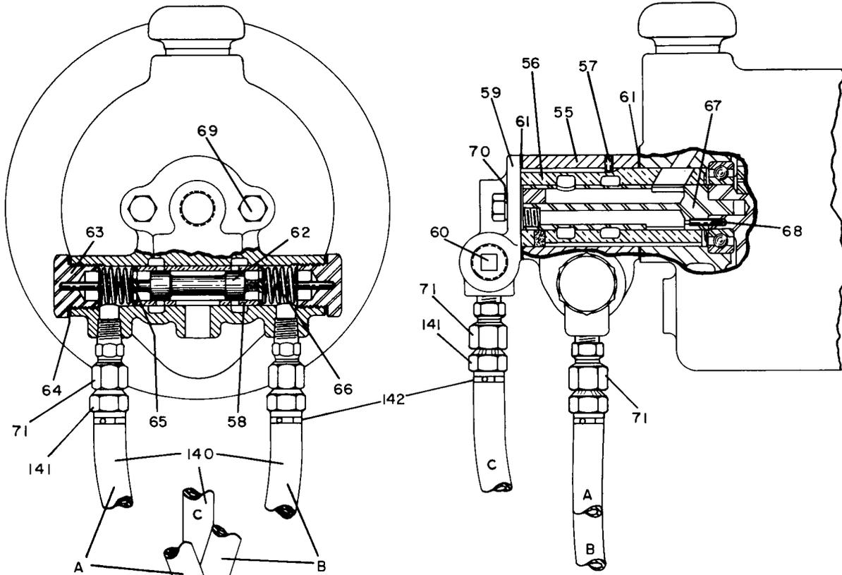
NOTE: IN ORDER THAT TROLLEY WILL MOVE TO LEFT WHEN THROTTLE LEVER ON LEFT OF PENDENT THROTTLE HANDLE IS PRESSED, AND MOVE TO RIGHT WHEN THROTTLE LEVER ON RIGHT IS PRESSED, HOSES A & B MUST BE CROSSED AS SHOWN BETWEEN HANDLE AND SHUTTLE VALVE CHEST.
